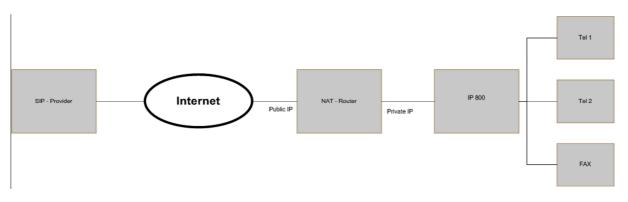
This scenario describes a setup where the PBX and phones are in a private network. The IP800 must use a stun server, in order to send correct SIP - messages. The IP800 works as media relay, all RTP - streams go through the PBX.
