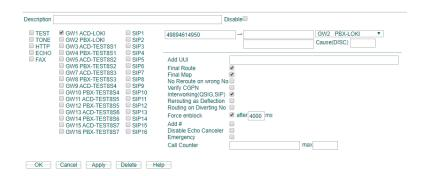
In the jtel ACD view, the property "Force enblock" must be absolutely activated in the Inbound-Route. Otherwise the calls in the by-election process will be sent to the jtel ACD. However, this by-election will no longer be considered or will be interpreted as DTMF input for IVR menus. In order to identify the respective service phone numbers in E164 format, the whole number in block will be needed.
