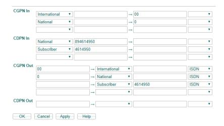
In the tab "Routes", phone numbers that should be transferred to the jtel ACD and those that Innovaphone should be handled internal are determined.
