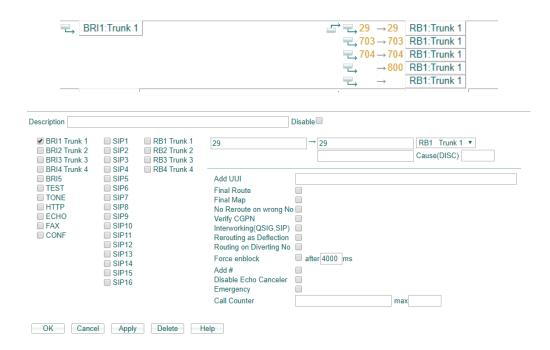
In the sample connection, the 800 within the Innovaphone PBX is used as routing for ACD objects. Therefore, the first three phone numbers (29, 703 and 704) are routed directly within the PBX, and all other incoming phone numbers are transferred to the jtel ACD.
