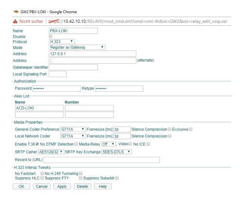
The PBX internal gatekeeper establishes a connection between office connectors and internal core processes. A corresponding entcryption 128-bit, format "SDES-DTLS", and the protocol H.323 will be set up. The local address of the PBX should be entered as IP address:
