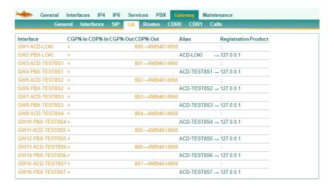
In our example the GKs GW1, GW3, GW5, GW7, GW9, GW11, GW13 and GW15 for which inbound calls, from the jtel ACD view, are used. The PBX sends calls to the respective ACD system throught these routes.
