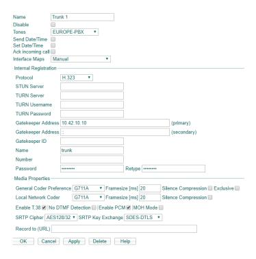
The name of the interface and the gatekeeper can be assigned independently. It is important that the gatekeeper address points at the Innovaphone PBX.
