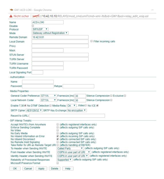
In the input field "Remote Domain" the respective IP address of the 8server, "test8s5" in this example, is entered.
