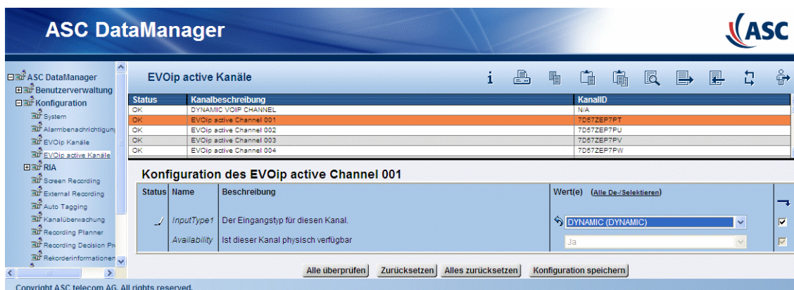
Abb. 8 - ASC DataManager: Menü Konfiguration - Konfiguration EVOip active Kanäle (EVOip active Channel)
